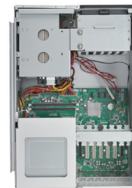
Easy-to-maintain power supply bracket
